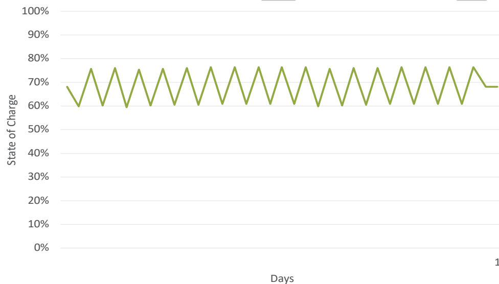
Figure 3 - Charge Sustaining Effect Starting at 70% SoC
