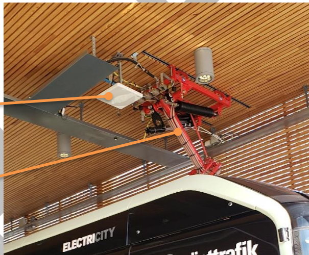
Figure E3 - Ceiling Mounted Overhead Pantograph
