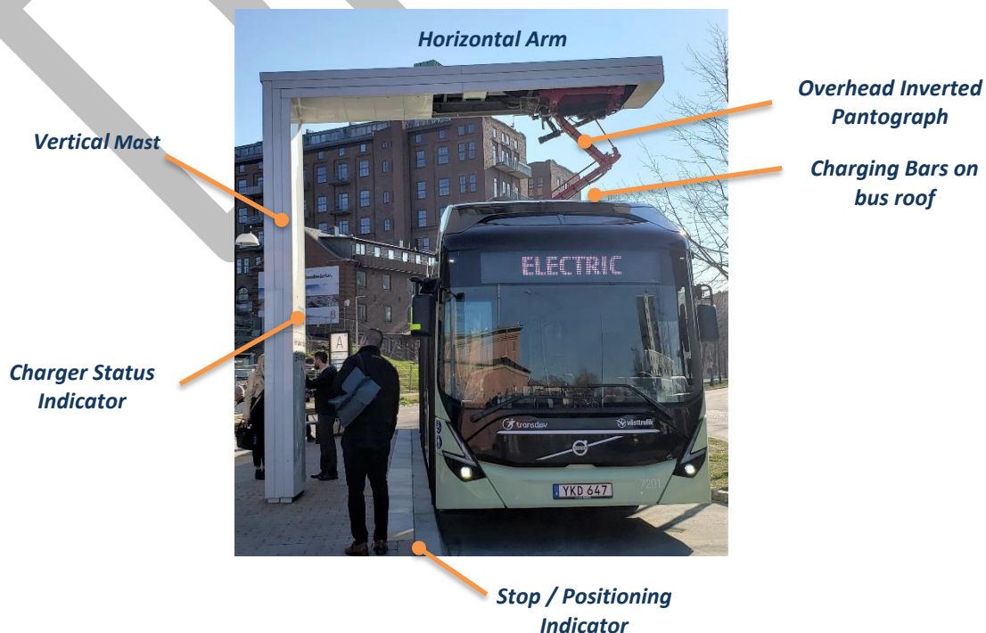
Figure 13 - Charging Mast and Components
