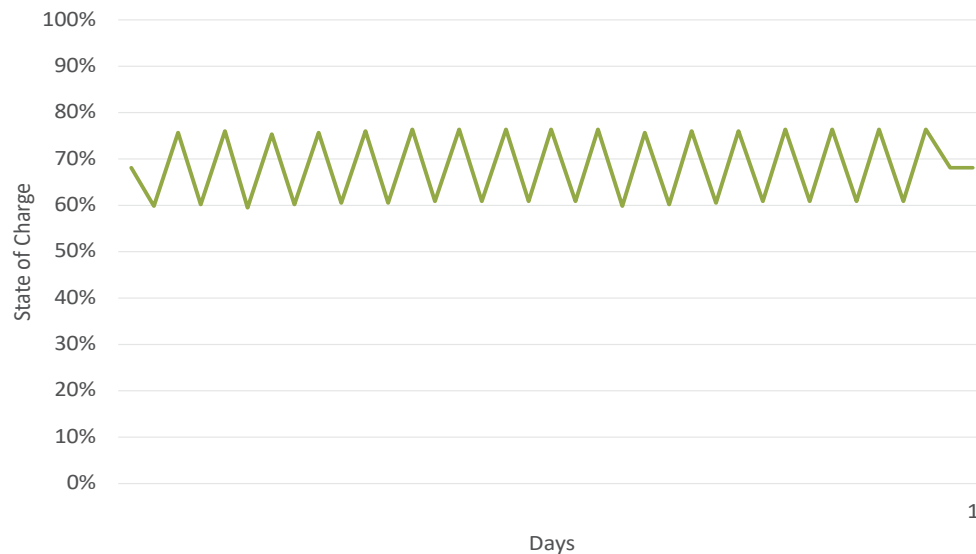
Figure 3 - Charge Sustaining Effect Starting at 70% SoC
